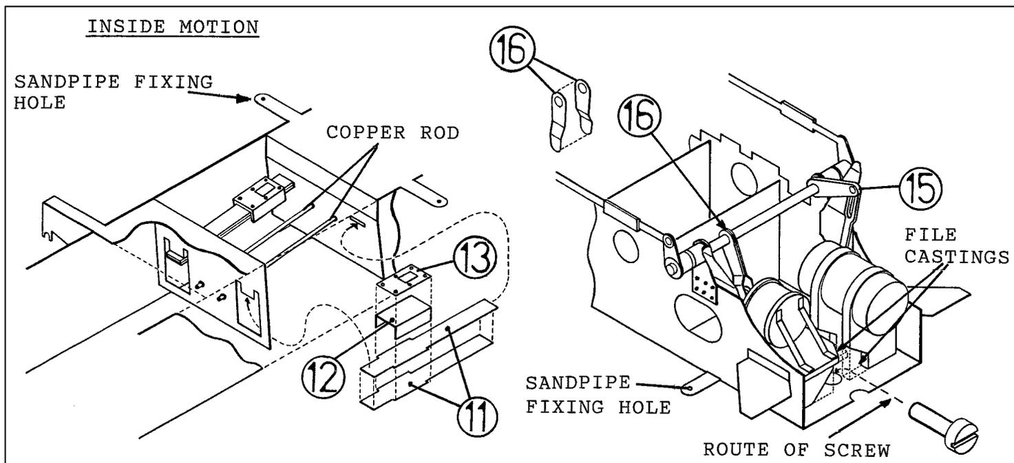
12) I have provided a representation of the top of the motion to go between the frames. Laminate slide bars together, parts 11, then make up the top of the crosshead from parts 12 & 13. Solder crosshead onto slidebars and then solder the front of the slidebars into the slot in spacer A. Solder the back of the slidebars to the top of the motion bracket, spacer C. Fit two lengths of 1.2mm copper rod through the central holes to represent the valve rods.
